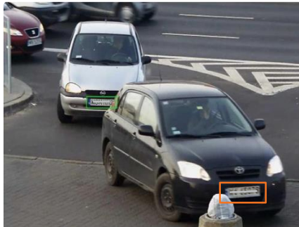
Depth of field is insufficient to cover foreground license plates. Adjust the lens settings.
