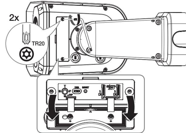
2. Insert a Micro SD card in the direction of the arrow.
