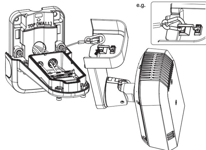
7. Attach the camera to the lower part of the mount using a screwdriver bit.
