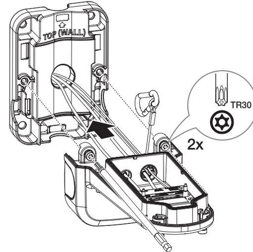
6. Connect the safety cable at the bottom of the mount to the hook at the top of the mount.
