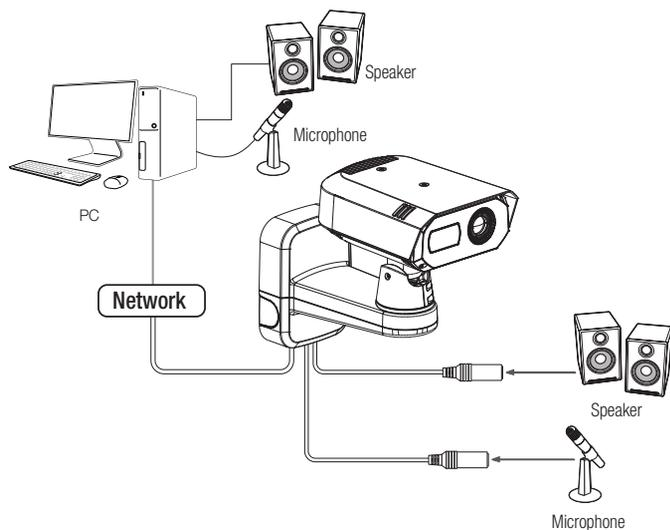
1. Connect the MIC terminal of the camera to a microphone or LINE OUT port of the amplifier where a microphone is connected.
