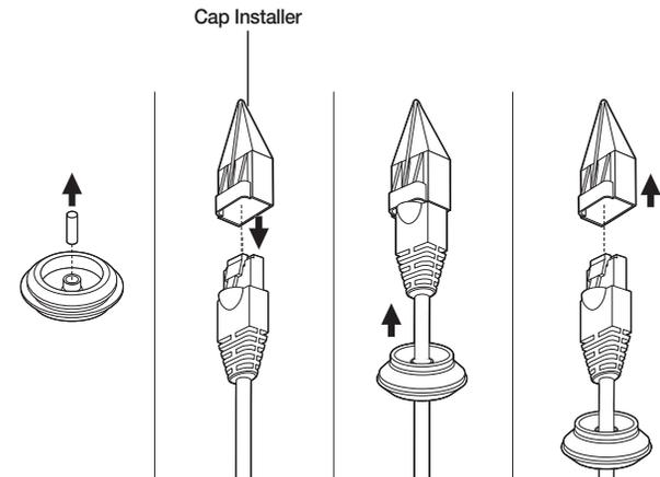
3-3. Connect the cable bushing with the network cable inserted into the lower part of the wall mount as shown in the figure.
