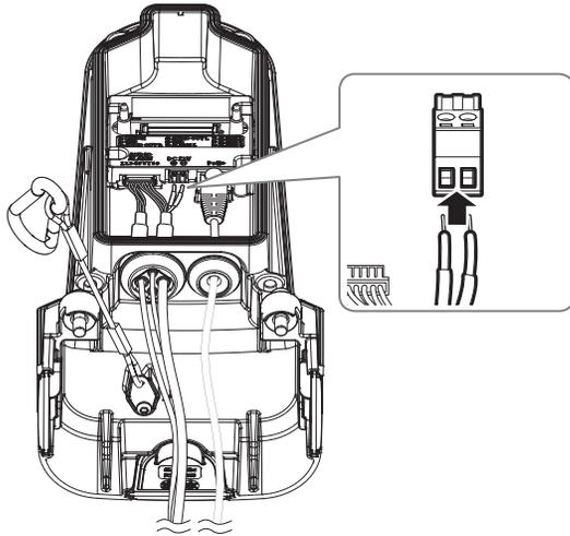
! ■ When connecting the power line to the power terminal block, paying attention to the polarity by referring to the imprint when connecting it.
