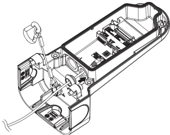
3-4. Connect the network cable's connector to the PoE+ connection terminal.
