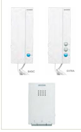
**LOFT:** Made of high-impact ABS with a texturised finish for easy cleaning and ultraviolet protection. It has many attachment points for wall mounting, as well a coiled cord with telephone plug connectors. A magnet located in the handset facilitates to hang it up correctly. Dimensions: 85x220x40mm
