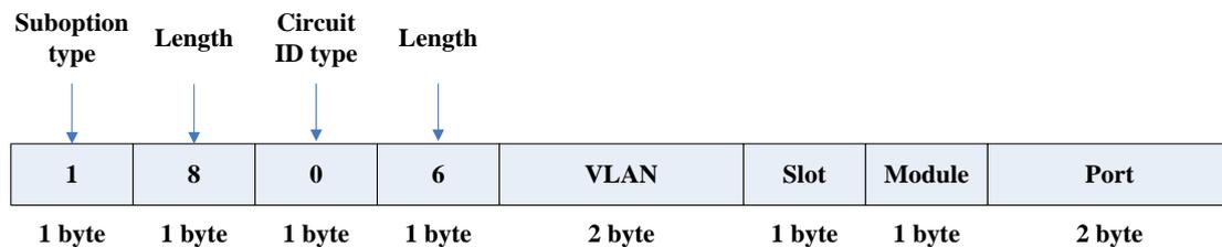
VLAN field fill in VLAN ID. For chassis switch, Slot means slot number, for box switch, Slot is 1; default Module is 0; Port means port number which begins from 1.
