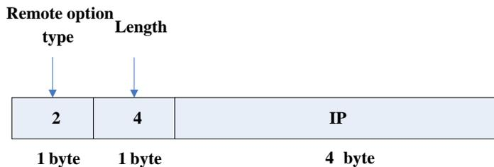
IP means the primary IP address of layer 3 interface where DHCP packets from.
