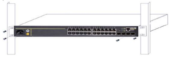
Fig 2-2 Fasten the Switch to the Rack
