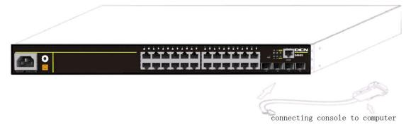
Fig 2-3 Connecting Console to switch
