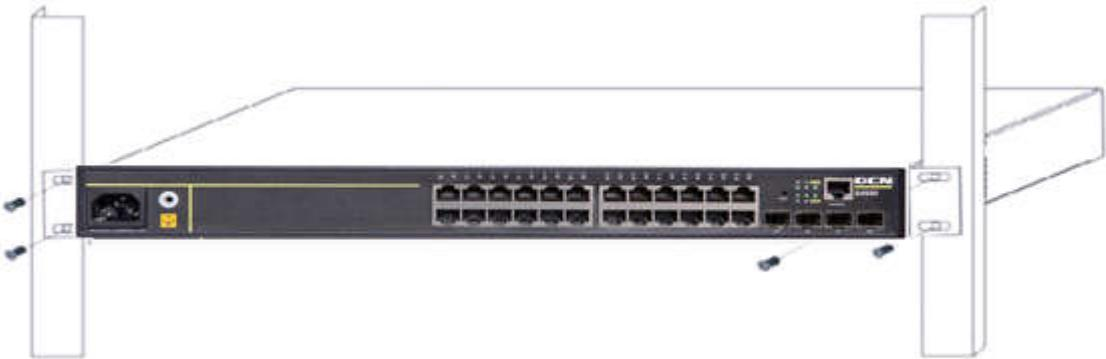
Fig 2-2 Fasten the Switch to the Rack
