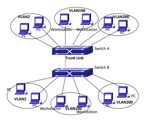
Figure 2-19 Typical VLAN Application Topology
