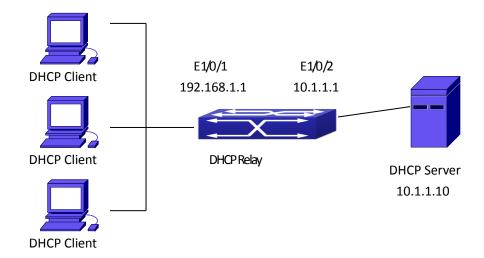
Figure 3-6 DHCP Relay Configuration
