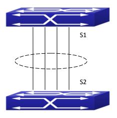
Figure 2-10 Configure Port Channel in LACP
