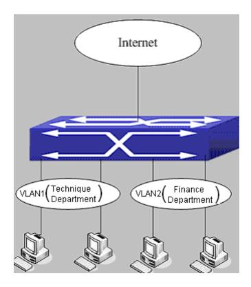
Figure 5-26 VLAN-ACL configuration example
