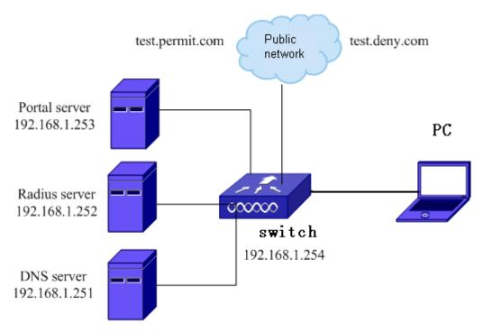
Figure 5-32 http-redirect-filter function case
