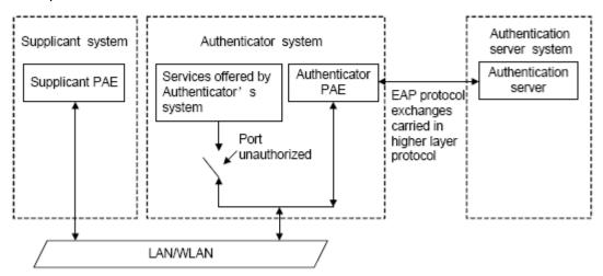
Figure 5-1 The Authentication Structure of 802.1x
