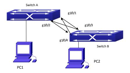
Figure 2-6 Fiber Cross Connection
