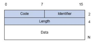
Figure 5-4 the Format of EAP Data Packets
