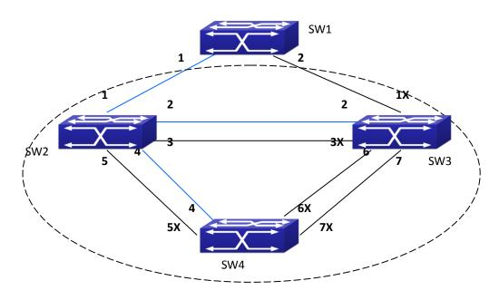
Figure 6-3 The Topology Of the Instance 0 after the MSTP Calculation
