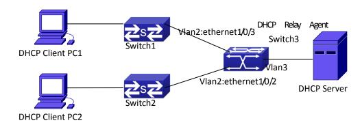
Figure 3-9 A DHCP option 82 typical application example
