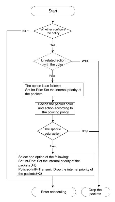
Figure 5-45 Policing and Remarking process
