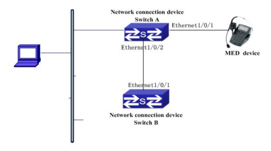
Figure 2-8 Basic LLDP-MED configuration topology
