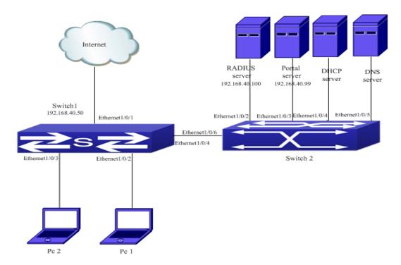
Figure 5-31 Automatic Page Pushing after Successful Authentication Configuration Configuration steps:
