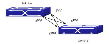
Figure 2-4 Fiber Cross Connection
