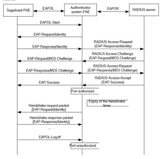
Figure 5-9 the Authentication Flow of 802.1x EAP-MD5
