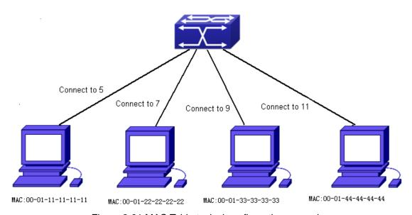
Figure 2-31 MAC Table typical configuration example
