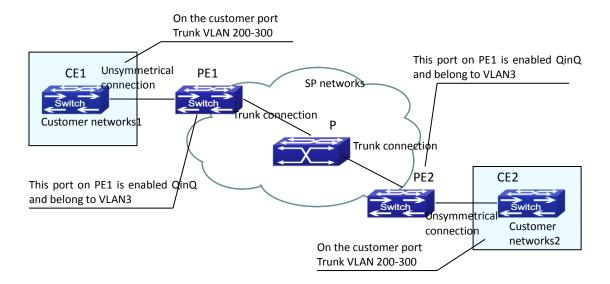
Figure 2-23 Dot1q-tunnel based Internetworking mode
