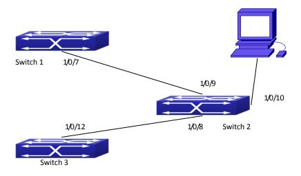
Figure 2-1 Port Configuration Example No VLAN has been configured in the switches, default VLAN1 is used.
