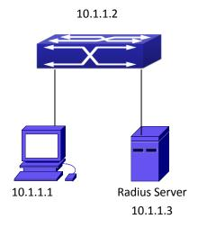
Figure 5-22 The Topology of IEEE802.1x configuration
