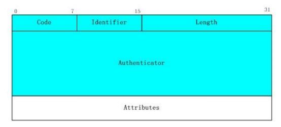
Figure 5-21 Message structure for RADIUS
