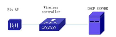
Figure 3-13 Typical DHCP option 60 and option 43 topology
