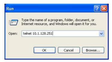
Figure 1-7 Run telnet client program included in Windows
