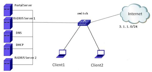
Figure 5-30 Authentication White-list function configuration
