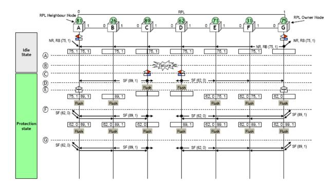
Figure 6-6 single-link fault
