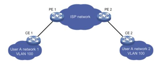
Figure 2-12 BPDU Tunnel application
