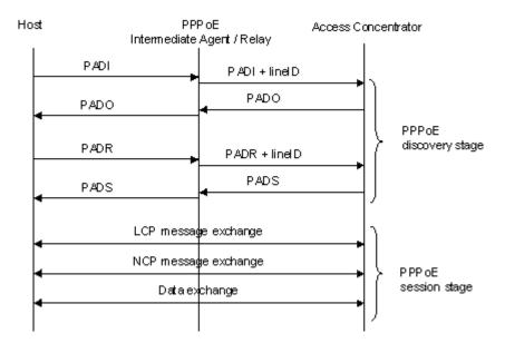
Figure 5-37 PoE IA protocol exchange process
