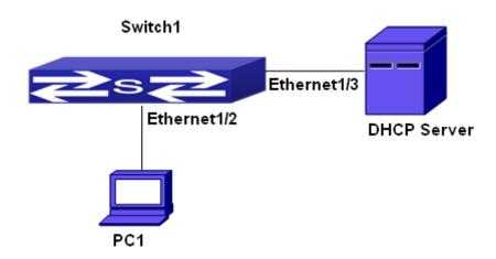
Figure 3-7 DHCP configuration example
