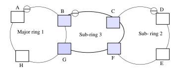
Figure 6-10 the interconnection ring topology without virtual channel
