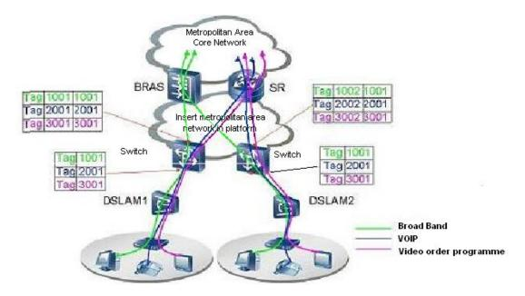
Figure 5-48 exible QinQ application topology
