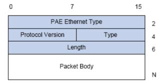
Figure 5-3 the Format of EAPOL Data Packet
