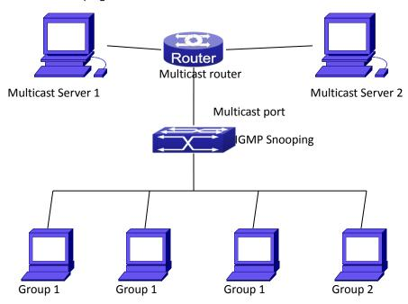
Figure 4-1 Enabling IGMP Snooping function
