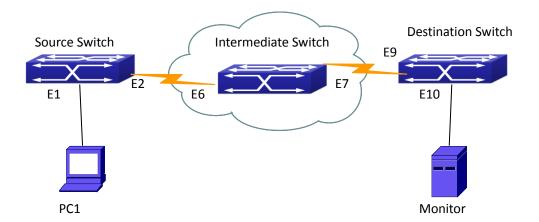
Figure 7-1 RSPAN Application Sample
