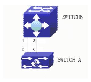
Figure 2-7 LLDP Function Typical Configuration Example
