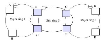
Figure 6-9 the interconnection ring topology with virtual channel
