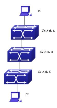
Figure 2-22 Typical GVRP Application Topology
