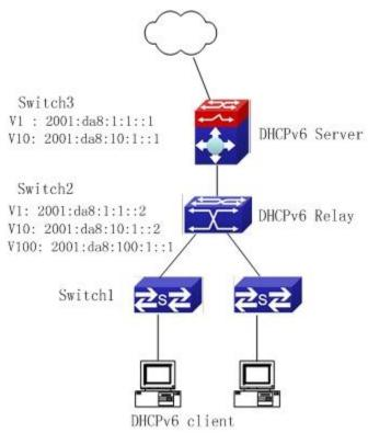
Figure 10-3 DHCPv6 relay option schematic
