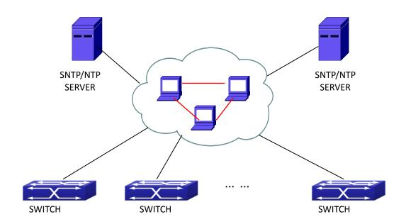
Figure 8-2 Typical SNTP Configuration
