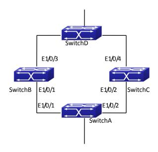
Figure 6-18 Fig 5-2 ULSM typical example
