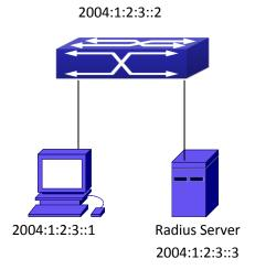
Figure 5-23 The Topology of IPv6 Radius configuration
